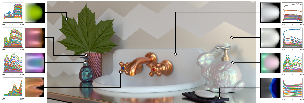
Figure 1: Spectral rendering of isotropic and anisotropic materials acquired from real-world samples using our method; insets show corresponding reflectance spectra. We measured these BRDFs using a motorized gonio-photometer; leveraging our novel adaptive parameterization to simultaneously handle BRDF acquisition, storage, and efficient Monte Carlo sample generation during rendering. Our representation requires 16 KiB of storage per spectral sample for isotropic materials and 544 KiB per spectral sample for anisotropic specimens.
