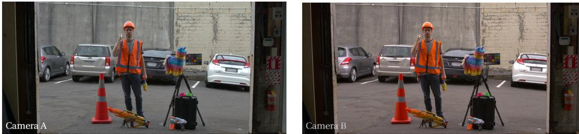
Figure 3.14: Camera A and B reproduction of an outdoor scene with their white-balance set to 6500K.
