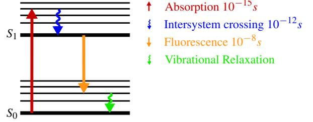
**Figure 2:** Jablonski diagram for fluorescence. Straight (wavy) lines represent radiative (nonradiative) transitions.
