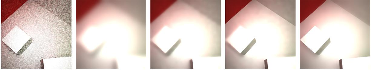
**Figure 4:** Å-Trous filter with increasing number of edge weights: unfiltered rt buffer (input), no additional weights: (“pure” Å-Trous ), rt buffer only:  $\sigma_{rt}$  (bilateral approx.), two buffers:  $\sigma_{rt}, \sigma_n$  and all three buffers:  $\sigma_{rt}, \sigma_n, \sigma_x$  (our result)
