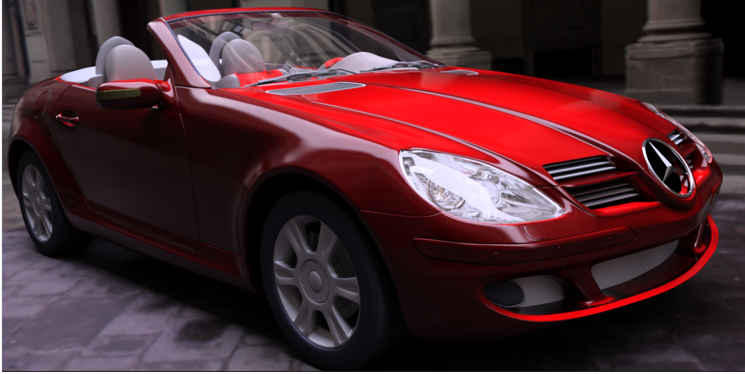
Figure 1.1: A car rendered using a ray tracing core completely based on fixed point arithmetic realized in integer arithmetic. To simplify custom shader writing, the color computations were performed using conventional floating point arithmetic. The quality of the fixed point computations is indistinguishable from computations in floating point arithmetic. Due to the equidistant spacing of fixed point numbers, the self-intersection problem can be tackled without a scene-dependent epsilon, which makes computations in fixed point arithmetic preferable.
