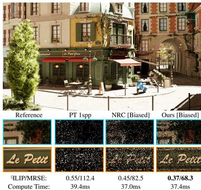
Figure 8: We present a comparative analysis of the performance between our Neural Incident Radiance Cache (NIRC) and the standard Neural Radiance Cache (NRC) when rendering the Bistro scene with environment lighting disabled on a RTX 3080 and path tracing (PT). It ensures a fair comparison since the standard NRC does not mitigate the variance caused by sky illumination estimation. The performance of both techniques is evaluated based on two metrics: Mean Relative Squared Error (MRSE) and \mathcal{F} LIP. It is evident from the results that despite its inherent bias, our NIRC estimator consistently outperforms the NRC in the provided scenario.
