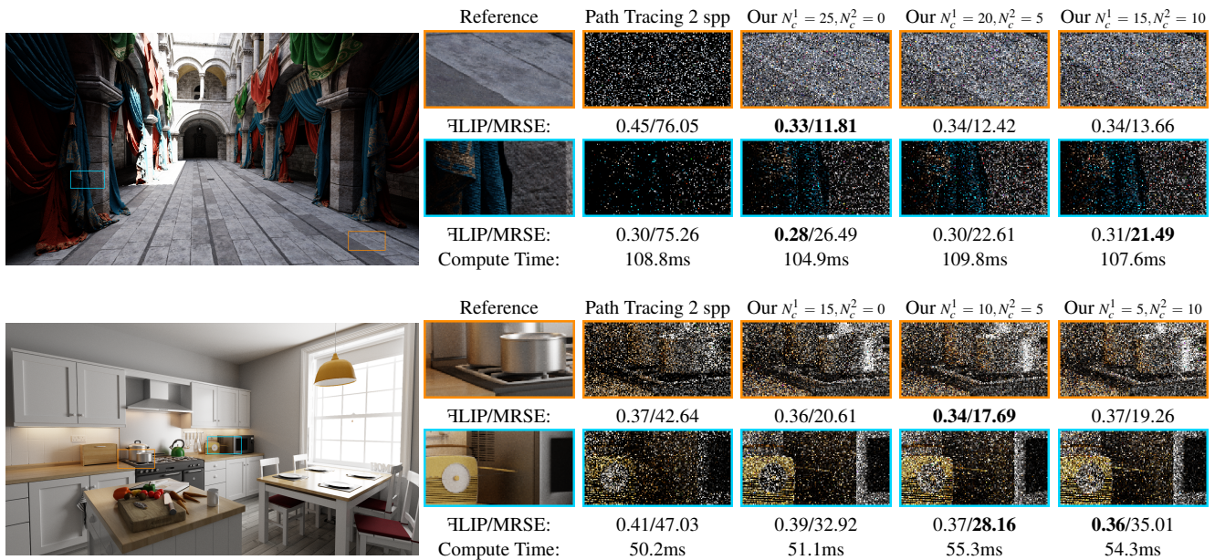
Figure 9: We explore the effect of redistribution of the number of neural samples between the first and second vertex of a light path, denoted as N_c^1 and N_c^2 , respectively. The experiments show the Sponza and Country Kitchen scenes rendered with up to 5 vertices in a light path without Russian roulette in order to match the render time. We observe that the optimal allocation of neural samples between the first and second vertex is highly scene-dependent, influenced by, for example, material properties and illumination.
